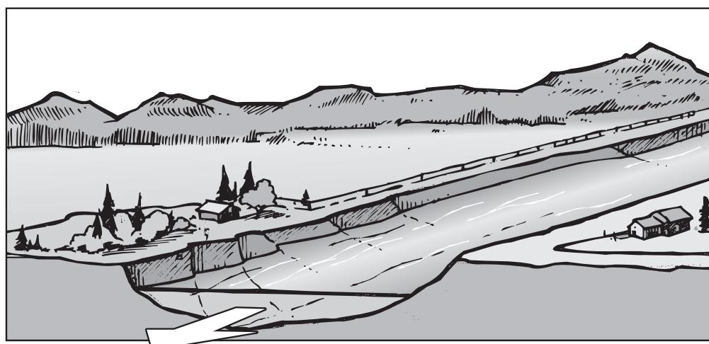
Fig 2-1 Laminar Flow in a smooth sided canal
