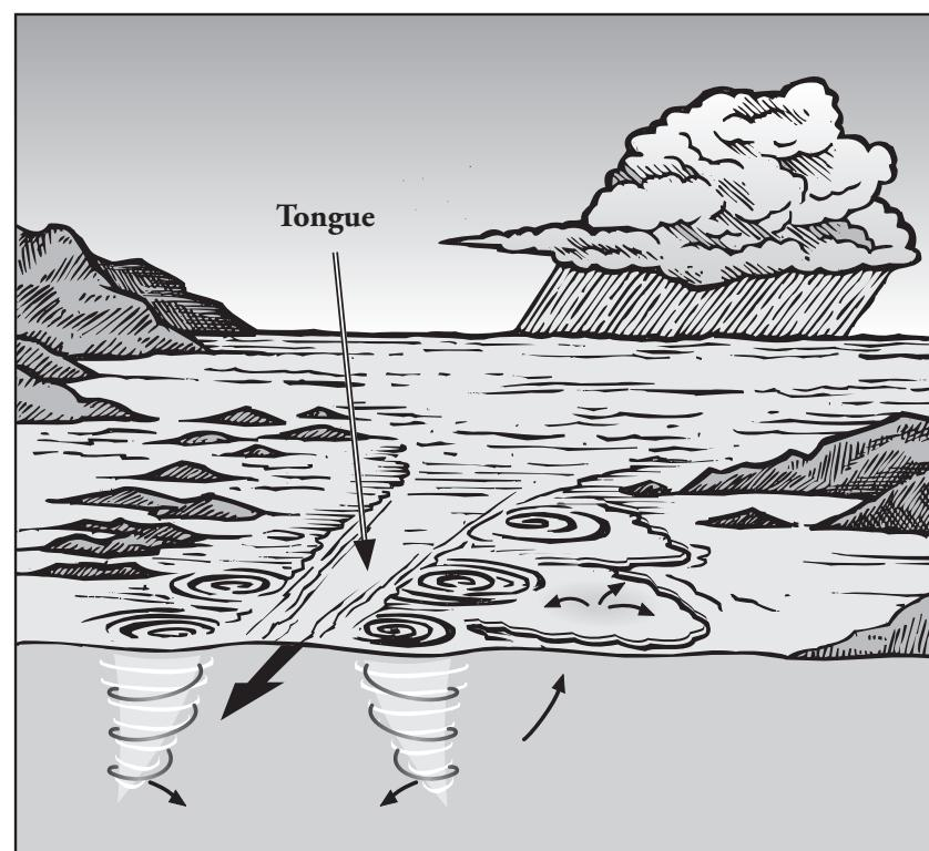
Fig 2-2 Subsidence (Whirlpools) and Upwelling (Boils) in a Tidal Rapids.
